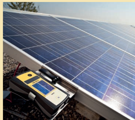
Install the TRI-SEN at the same level as the modules and measure the irradiation.
