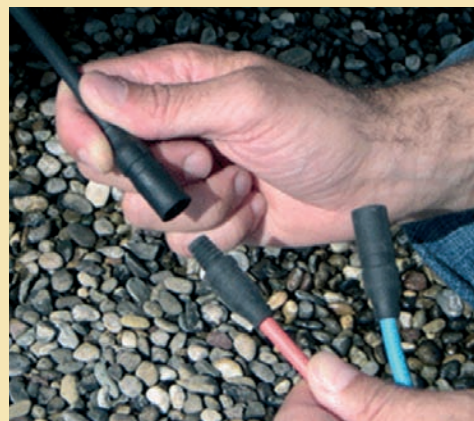
Disconnect loads from the solar modules and connect the TRI-KA to solar modules.
